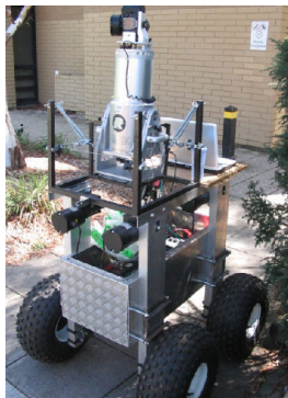
Fig. 2. Riegl LMS-Z420i Terrestrial Laser Scanner equipped with a calibrated Nikon D100 6 Mega Pixel digital camera
